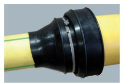
3. Pull integrally moulded sleeve collar over the casing pipe (sleeve can be stretched about 10 %) and attach the sleeve to the casing pipe with the larger of the straps included in the delivery.
