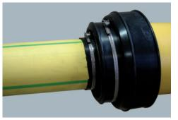
4. Wrap the annular space with the conical part of the S-shaped sleeve and attach it to the carrier pipe with the second strap.
