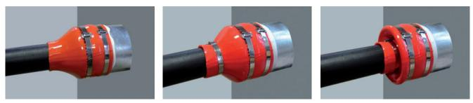
**4.** Align the sleeve on the carrier pipe elongated (figure a) or S-shaped (figure b) depending on the extension direction. Then install the first strap about 15mm away from the rear end.
