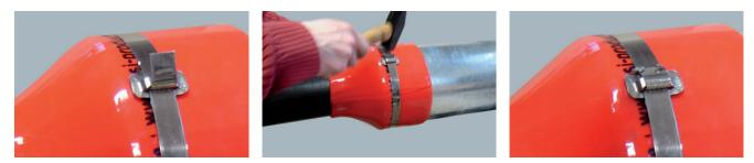
**4.** Cut off the steel strap with the clamping tool cutting lever to immediately obtain the correct length. Immediately strike the cut off end on the stainless steel loop with a hammer. Then bend over both barbs of the loop to protect the strap.
